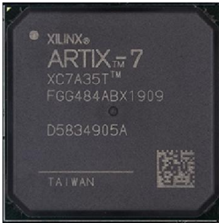
Figure 2-2: FPGA chip on board
