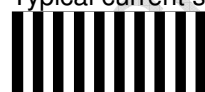
Fig2. Max current situation: Vertical stripe pattern alternating 0 gray scale with 255 gray scale every dot
